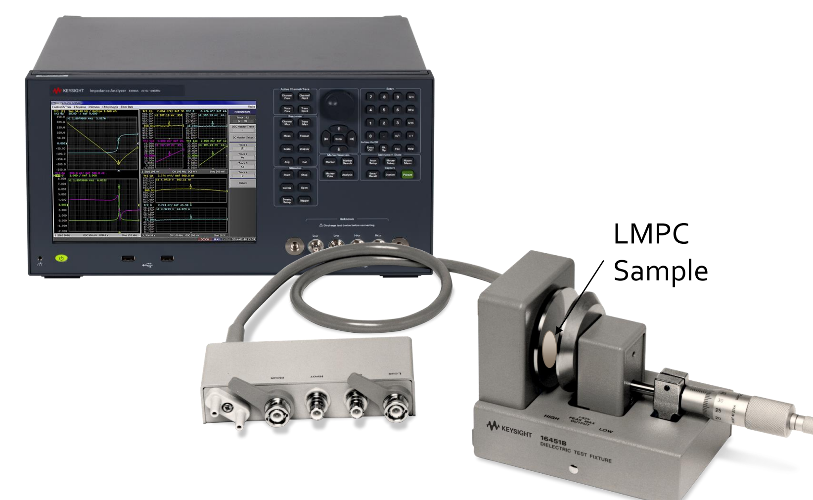
Figure 4: Electrical properties of PDMS were measured with an impedance analyzer and dielectric test fixture.
